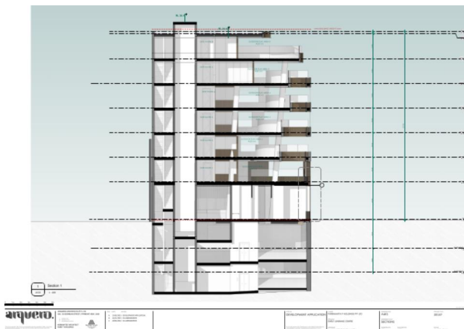
Figure 6: Section plan of the proposed child care centre.
